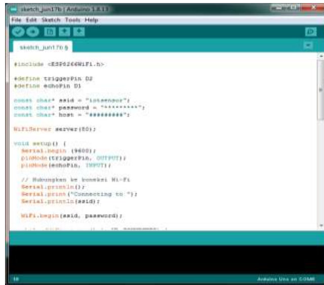
Figure 4. Internet network connection configuration via Wi-Fi on Arduino IDE
